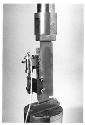
FIG. 3 Compressive Plate Shear Test
