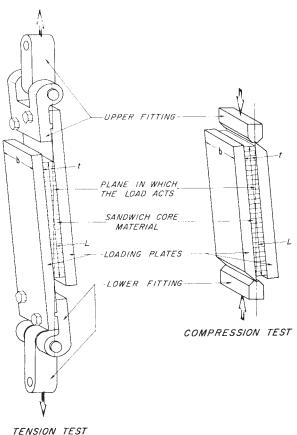
FIG. 1 Plate Shear Specimens, Load Line of Action
